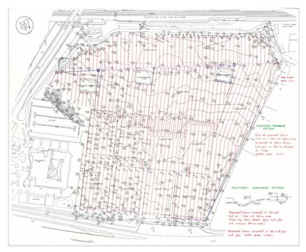
3.5 The second plan (Drawing No. XEV002-DR2) also shows the completed scheme without levels but also includes the drainage outlets in the south west corner and North east corner, and pipe sizes which vary between 60mm and 250mm.
