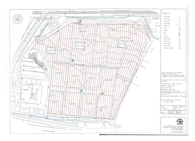
3.6 The drainage scheme is extensive and covers the whole field, with drainage runs at approximately 8m centres (note the attached plans are not to scale). Due to this coverage PCC do not consider that adequate consideration has been given to the time required for and complexity of reinstatement of the drainage system within the applicant's indicative timetable.
